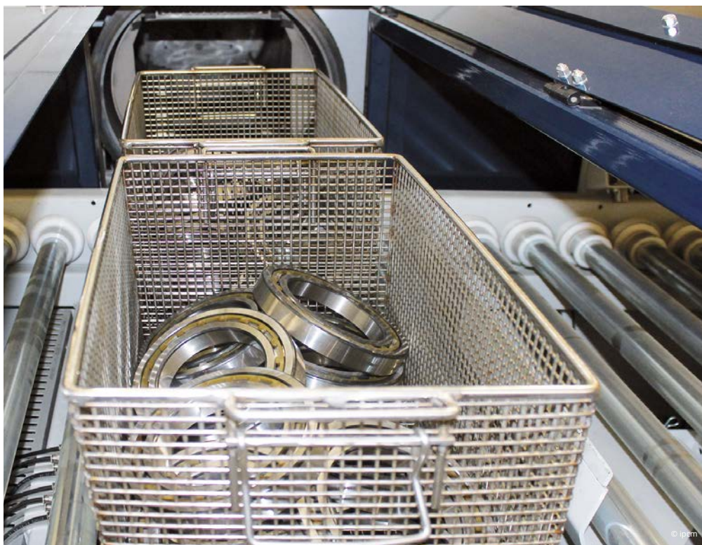
The inside of the IK40-e cleaning system and bearings placed in the basket before the cleaning operation.
