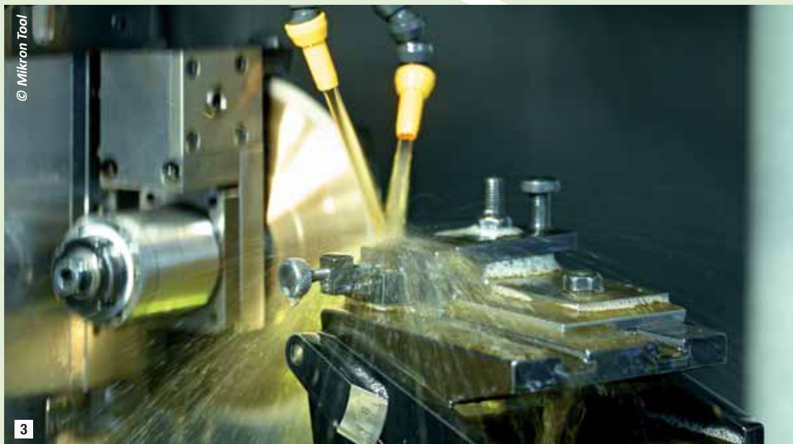
3 The grinding stage of the cemented carbide cylindrical bars: Grinding gives to the tool its geometrical shape by removing the excess material.
