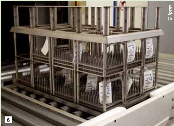
6 The 24 cleaning baskets have been standardized in order to contain the whole Mikron Tool production range. This standardization eased the adjustment of the cleaning process, which can vary only in two aspects: The switching off of the ultrasounds when the smallest and most delicate tools are cleaned, and the lacking of baskets tilting when the bigger tools are cleaned.
