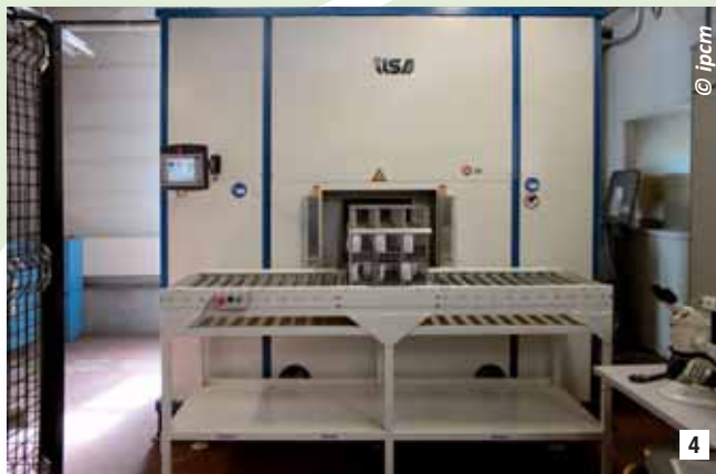
4 The vacuum closed-circuit cleaning system using modified alcohols was designed and manufactured by ILSA in San Vincenzo di Galliera (BO, Italy)
