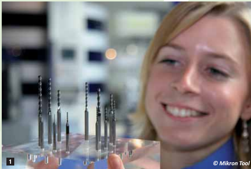
1 Mikron Tool manufactures tips, milling cutters, reamers, chamfering and deburring tools in cemented carbide with a diameter range from 0.1 to 32 mm.
