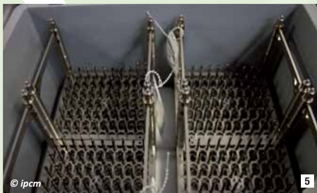
5 Mikron Tool did a very good study of the cleaning baskets so as to clean all the tools, included the biggest one, in a positioned fashion, with a higher quality and without the risk of damage
