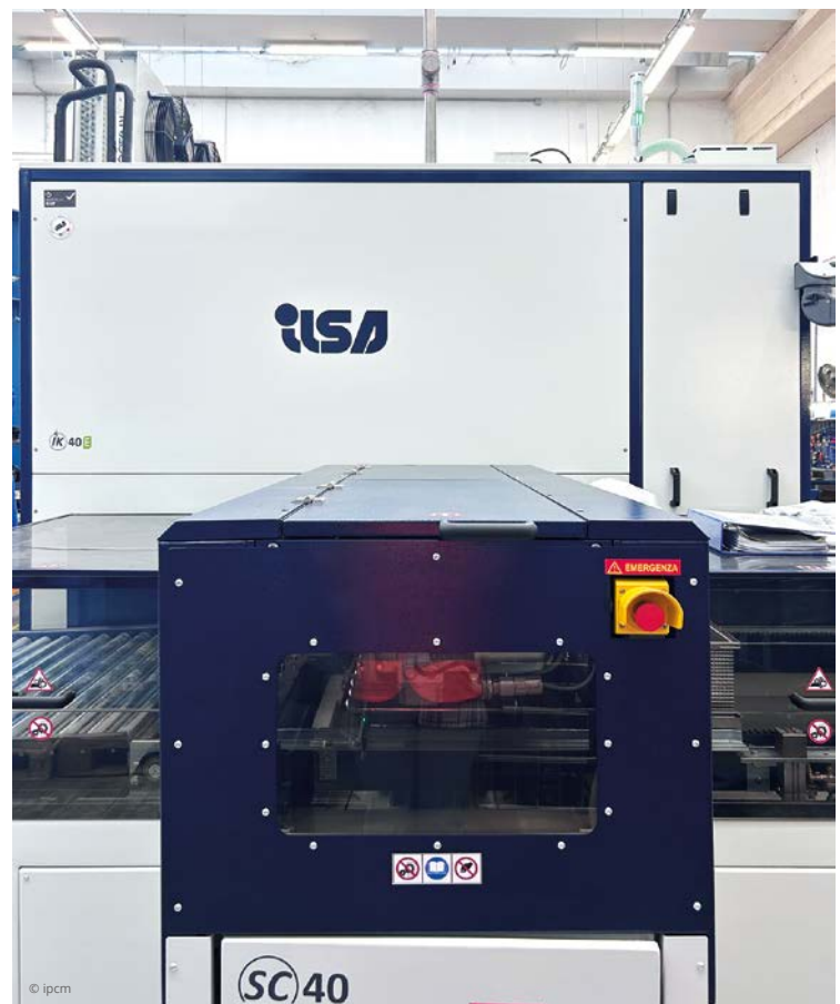
The closed-loop cleaning system operating under vacuum and using modified alcohol, designed and supplied by ILSA-MC.
