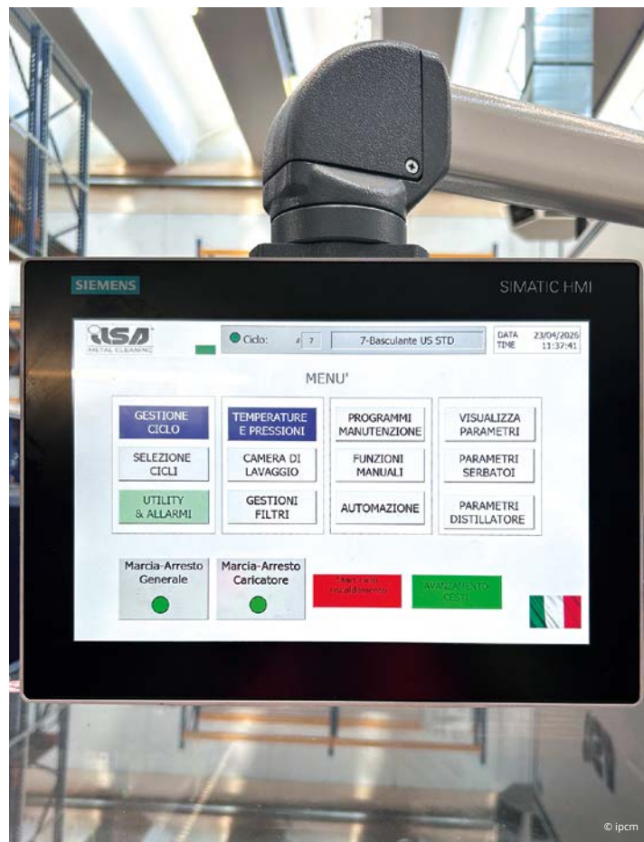
The touch screen of the machine. Each load can be assigned to a different cleaning cycle depending on the components’ specifications.
