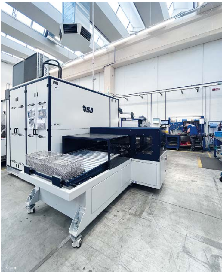
The closed-loop cleaning system operating under vacuum and using modified alcohol, designed and supplied by ILSA-MC.
